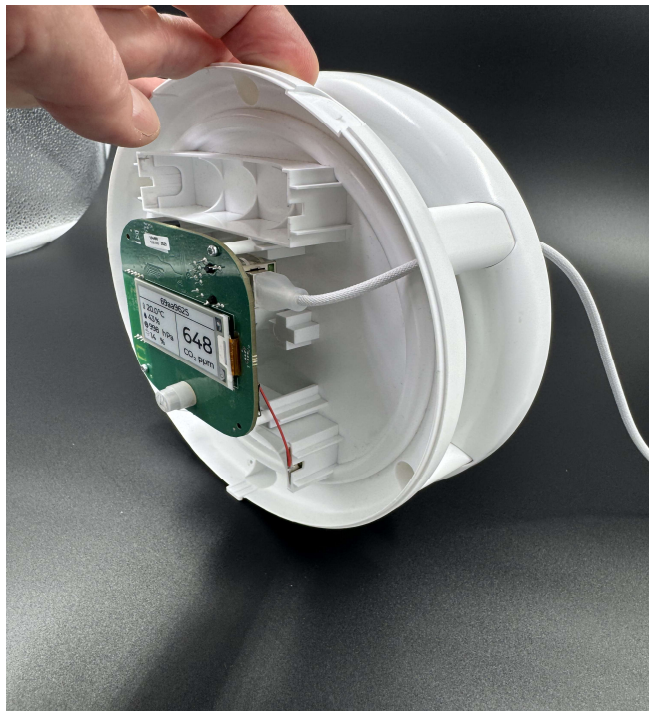
Figure 4 — Cable routed and valve ready for mounting.
