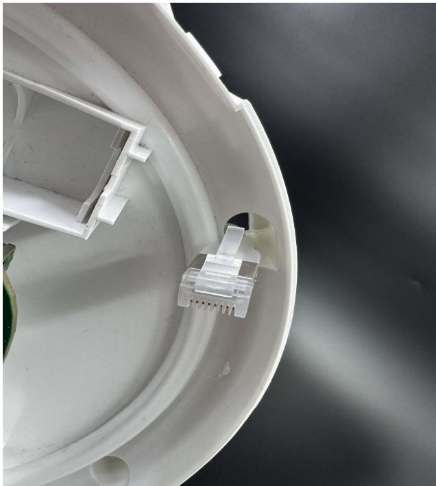
Figure 2 — Channel after opening, ready for cable insertion.
