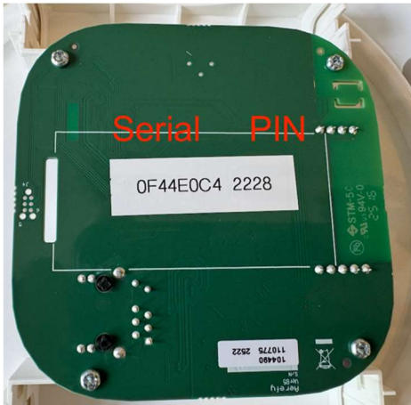
Figure 5 — Locating Serial no and PIN with the valves w/o display
